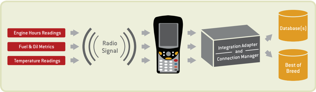
Figure 1. Example of RFID Information in Preventive Maintenance
